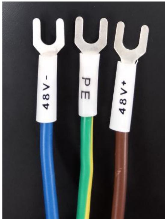
Figure 3 Definition of power line wires
