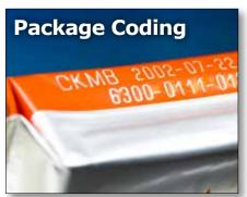
Easily applies permanent alpha numeric codes, barcodes, text, and expiration dates to a variety of packaging materials that will not smear or rub off.
