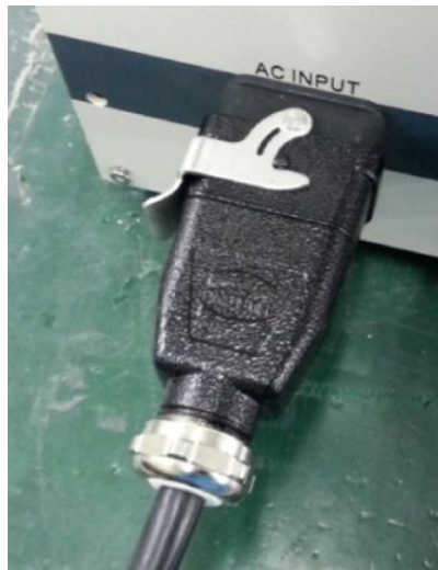
Figure 9 Lock the Plug with the Lever
