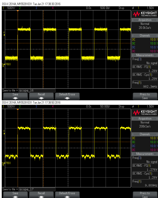
Figure 3a. Typical CW Ø1.5mm laser beam modulation oscilograms at 1Hz and 10Hz rates.
