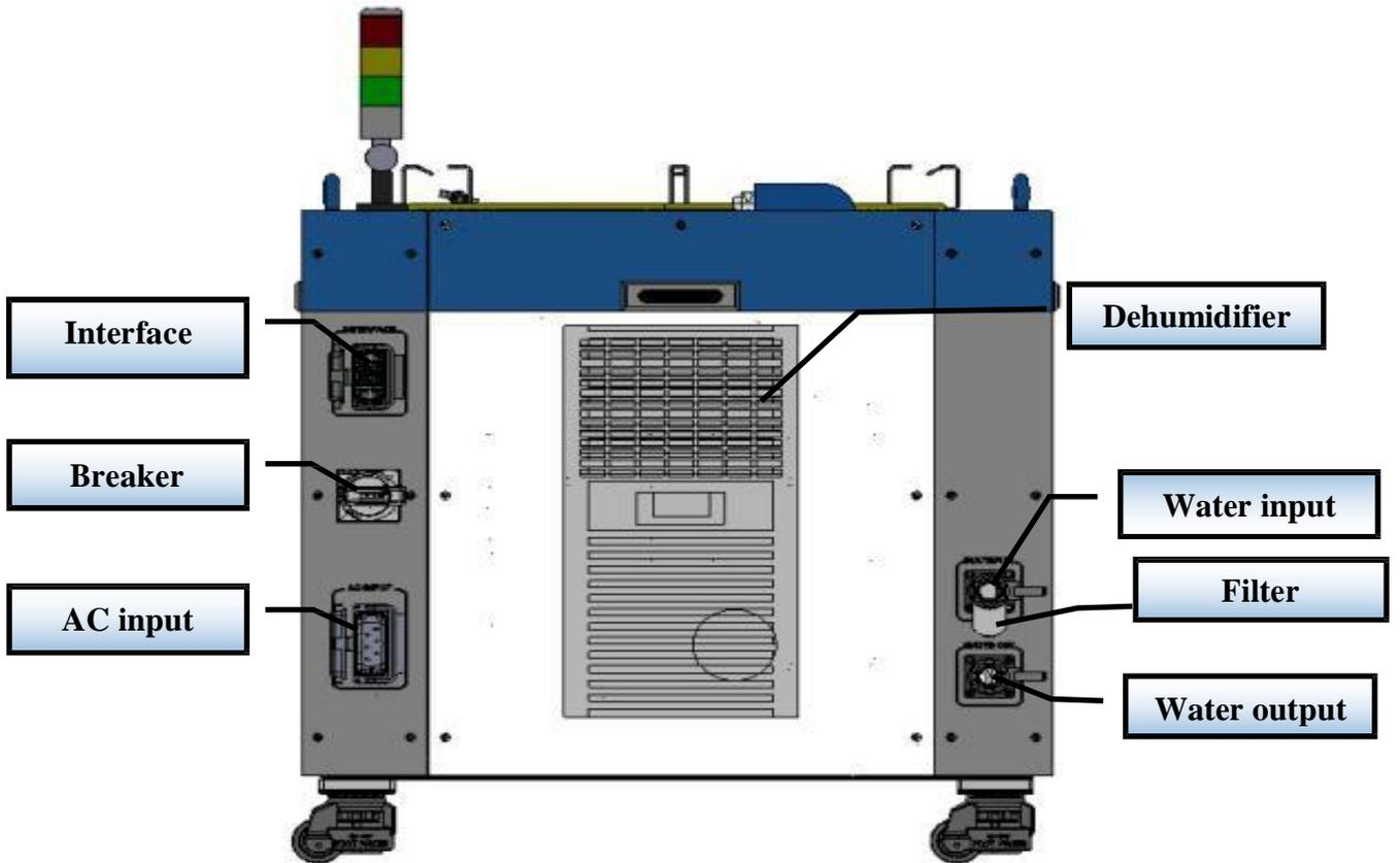
Picture 9-c Rear view of C10kW/C12kW product panel.
