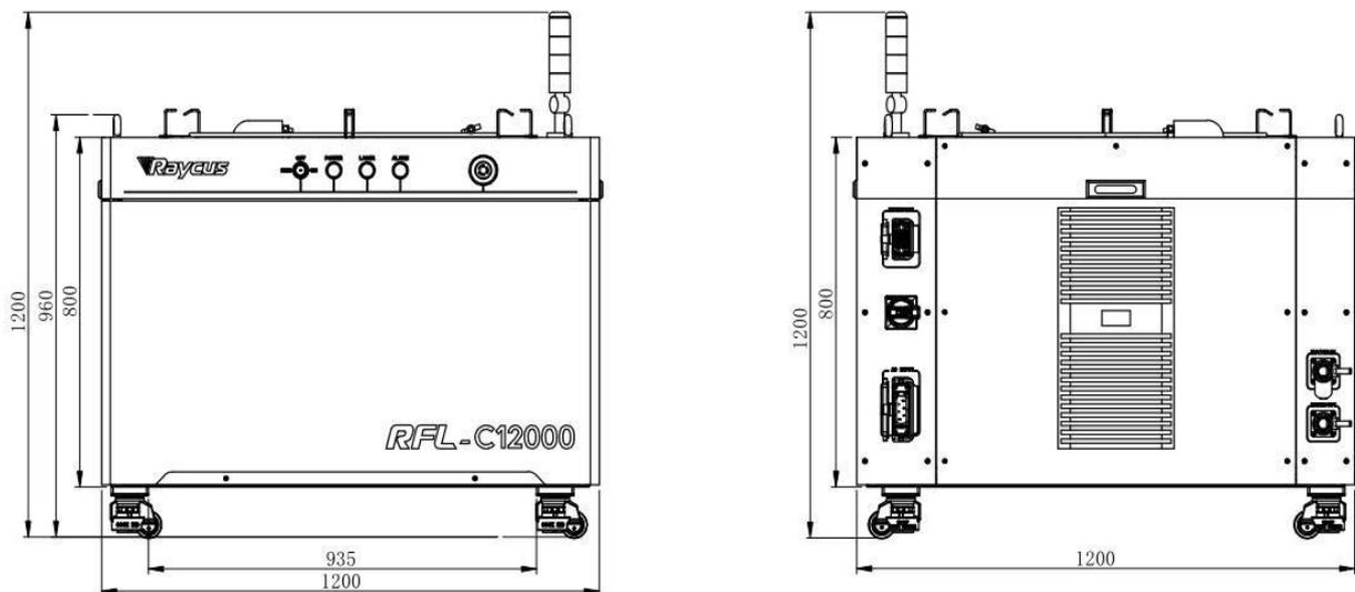
Figure 3-a Front and rear view of the laser
