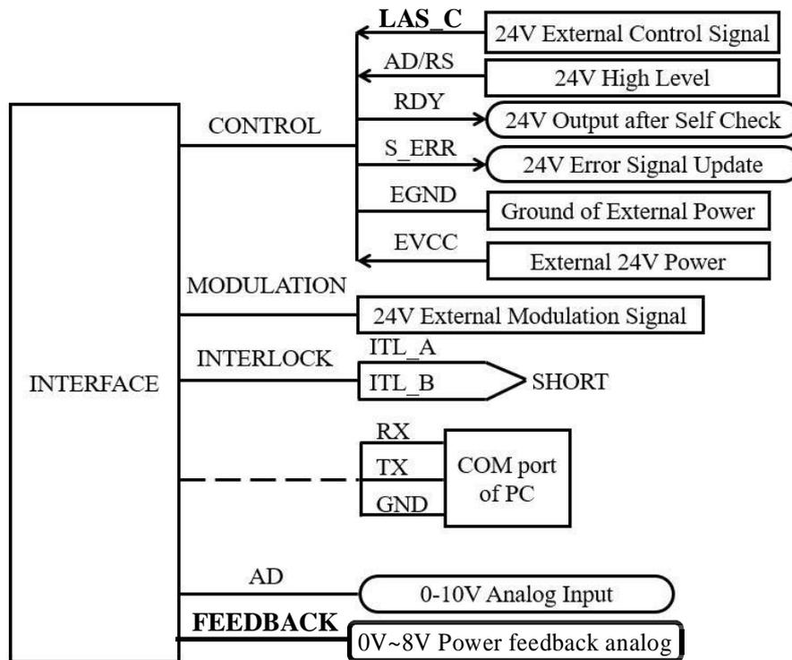
Figure 15 Wiring of Serial Port Communication Mode
