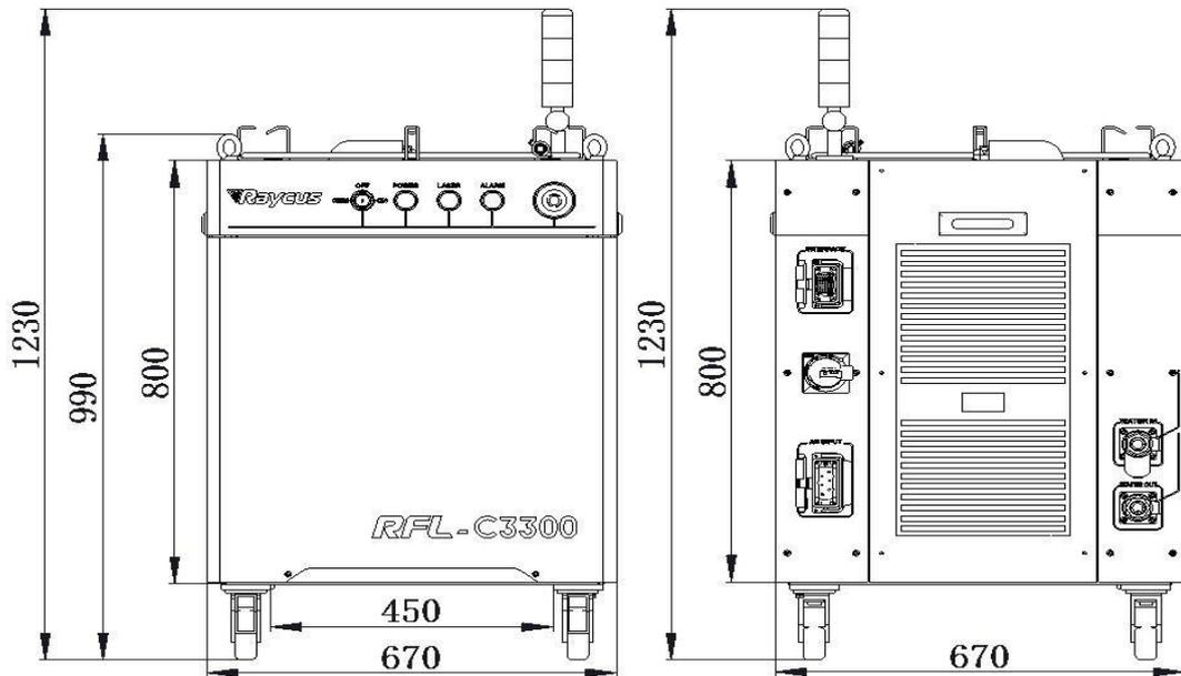
Figure 1-a Front and rear view of the laser.
