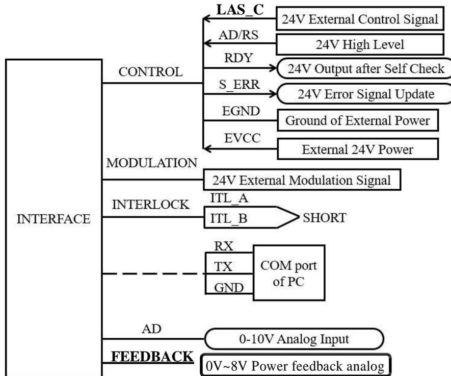
Figure 20 Wiring Diagram in AD mode.
