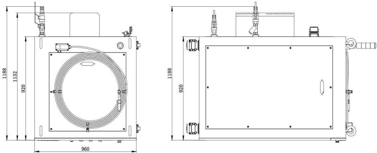
Figure 4-b Top and left view of the laser.
