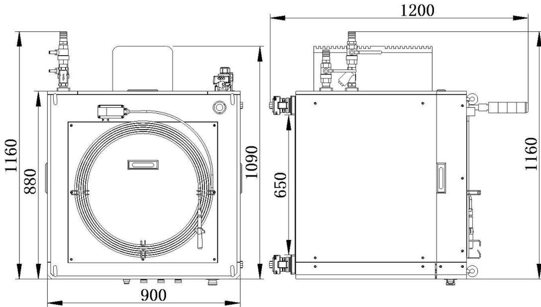
Figure 2-b Top and left view of the laser.
