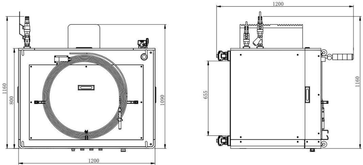
Figure 3-b Top and left view of the laser.
