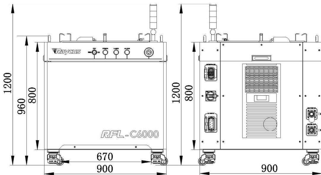
Figure 2-a Front and rear view of the laser.
